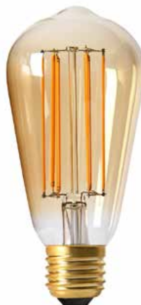
Code: LED-ST64-33 Dimension: Ø 64 mm, H 124 mm LED 4 Watt, 2000 Kelvin, 220lm Dimmable
